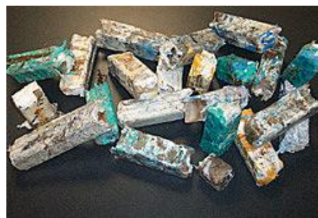
Figure 9. International Paper fuel cubes, made from compressed waste.
